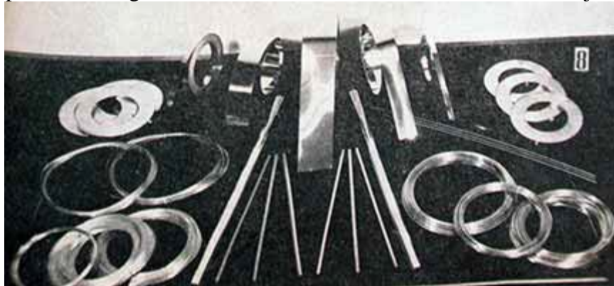
Figure 11 - Gold filled sheets, tubes, and wires ready to be sent to the jewelry manufacturer. Jewelry, September 1953.
